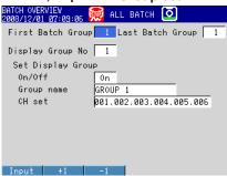
Press **MENU** (to switch to setting mode), and select the **Multi batch** tab > **Group set, Trip line** > **Trip line**.
