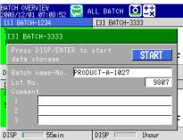
4. Use the arrow keys to move the cursor to START, and press DISP/ENTER. Recording starts for the selected batch group.
