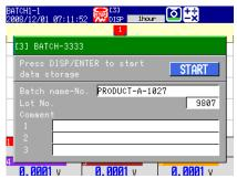
**3.** Use the **arrow keys** to move the cursor to **START**, and press **DISP/ENTER**. Recording starts for the batch group.
